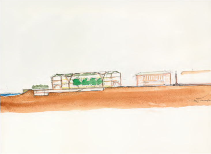
Tunnel section showing the traffic at the lower level and the connections between the museum and the upper tunnel. The sculpture garden on the surface and the steps of the pier are also shown
